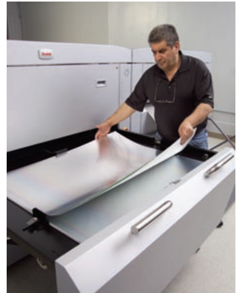
Platesetter operator Ghazi Halloum loads a Sword Excel plate into the Magnus 800 platesetter.
