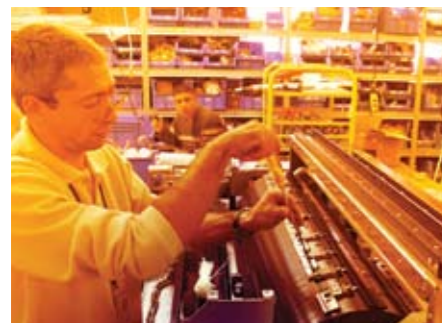
Replacing and aligning drum grippers
