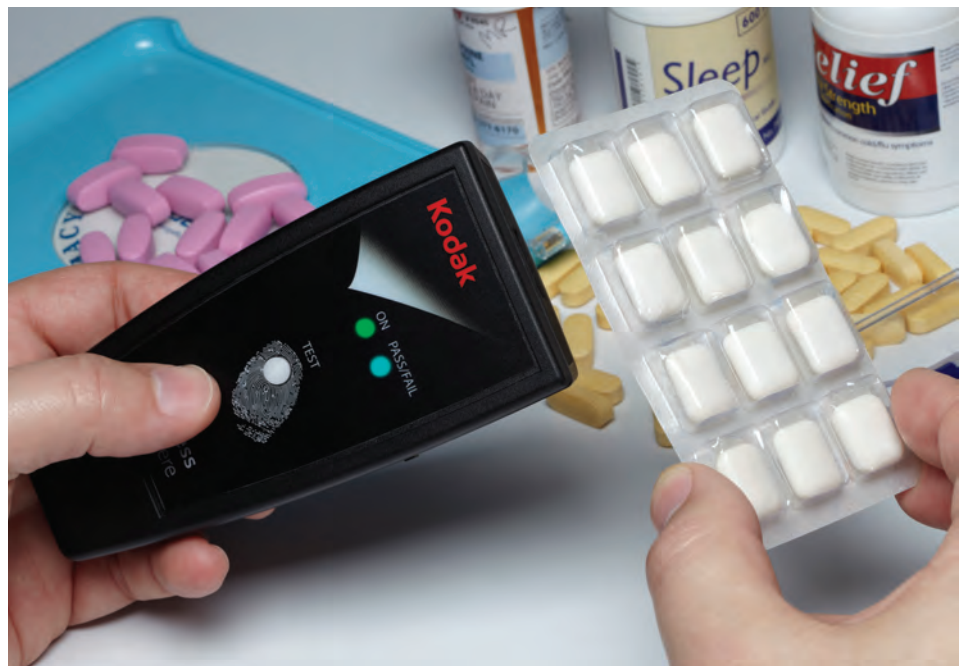
The Kodak Traceless Anywhere System, capable of invisible authentication on paper, inks, toners, coatings, paints, fabrics, fibers, plastics, foils, and glass.
